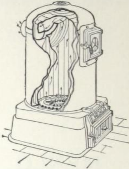
Nos. 10, 12 and 14 Menlo Showing Fire Travel
